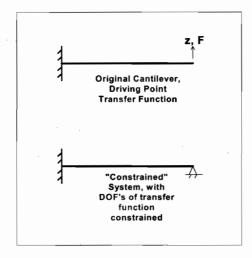
Figure 4.10: Unconstrained and constrained cantilevers used for driving point transfer function example.
