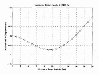
Figure 14.3: Cantilever beam second mode.
