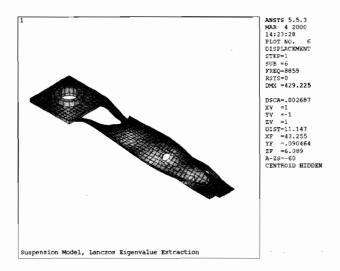
Figure 17.9: Mode 6, 8859 hz, second torsion mode.
