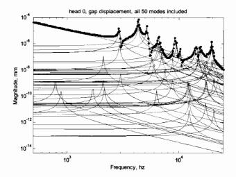
Figure 17.34: Head 0 frequency response, overlay of individual mode contributions, 50 modes included, uniform damping with zeta = 0.005.
