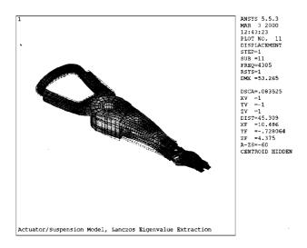
Figure 17.22: Mode 11 mode shape plot, 4305 hz, system mode.
