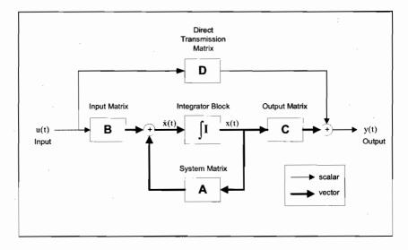
Figure A2.1: State space block diagram.
