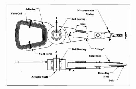
Figure 19.1: Drawing of actuator/suspension system.
