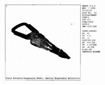
Figure 19.17: Mode 12, 3415 hz, suspension torsion, arm tip lateral.
