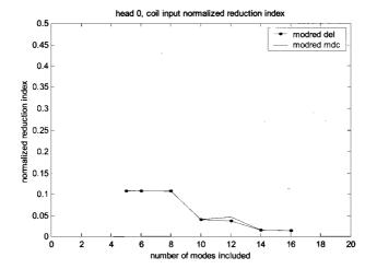
Figure 19.60: Head 0 impulse response normalized error index comparison for reduced modred models using "del" and "mdc" methods, coil input.
