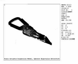
Figure 19.11: Mode 3, 1004 hz, arm/coil bending in phase.
