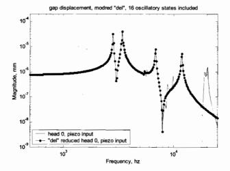
Figure 19.51: Head 0, piezo input, 16 reduced oscillatory states included.
