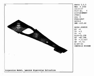
Figure 17.8: Mode 5, 6937 hz, sway or lateral mode.
