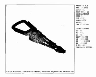
Figure 19.18: Mode 13, 3479 hz, coil/arm/suspension lateral mode.
