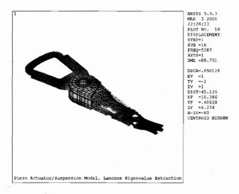
Figure 19.19: Mode 16, 5387 hz, suspension sway, arm tip lateral.
