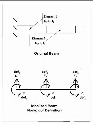
Figure 13.3: Two-element cantilever beam model and node definition.
