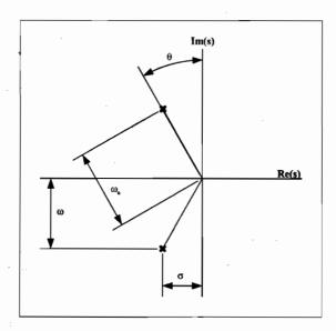
Figure 5.3: Complex eigenvalue (pole) nomenclature in complex plane.
