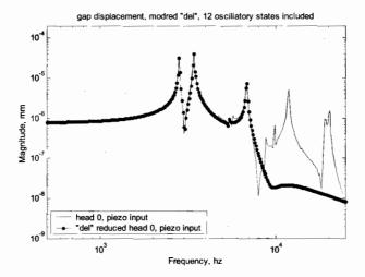
Figure 19.47: Head 0, piezo input, 12 reduced oscillatory states included.
