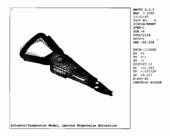
Figure 17.19: Mode 6 mode shape plot, 2114 hz, coil torsion.
