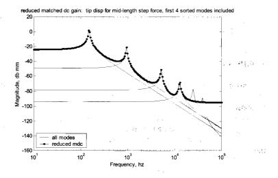
Figure 15.18: Cantilever tip displacement for mid-length force, first four sorted modes, "modred" "mdc" option.
