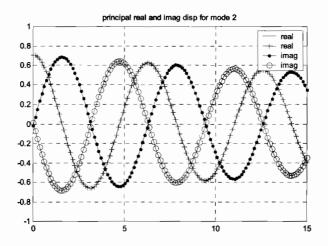
Figure 10.6: Principal real and imaginary displacements, mode 2.
