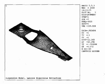
Figure 17.6: Mode 3, 3020 hz, first torsion mode.
