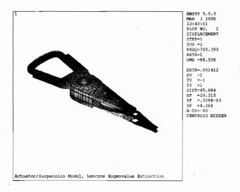
Figure 17.17: Mode 2 mode shape plot, 785 hz. Bending of bottom arm.
