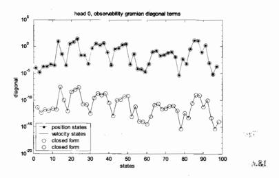
Figure 18.7: Observability gramian diagonal position and velocity state terms.
