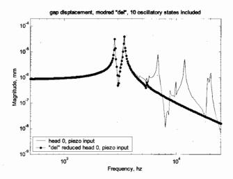
Figure 19.45: Head 0, piezo input, 10 reduced oscillatory states included.
