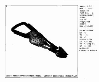
Figure 19.15: Mode 8, 2823 hz, suspension torsion, in phase, arm tip interaction.
