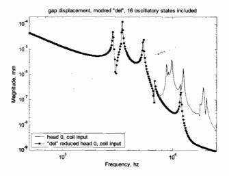
Figure 19.50: Head 0, coil input, 16 reduced oscillatory states included.
