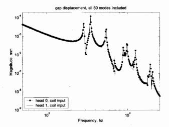
Figure 19.30: Frequency response for coil input for both heads, all modes included.
