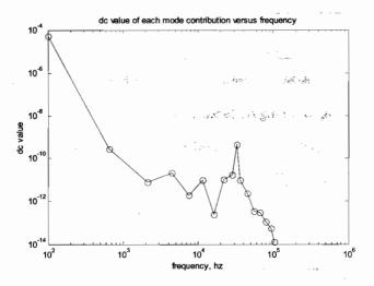
Figure 16.8: Low frequency and dc gain versus frequency.
