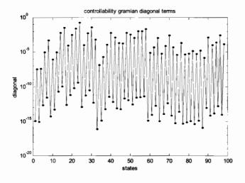
Figure 19.35: Controllability gramian diagonal terms versus states.
