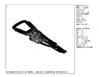
Figure 17.23: Mode 12 mode shape plot, 4320 hz, radial mode.
