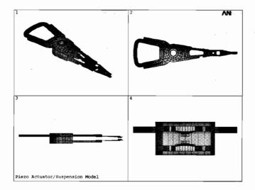
Figure 19.3: Piezo actuator/suspension model, four views.
