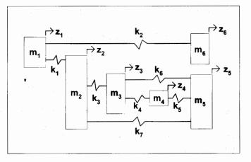
Figure 2.2: 6dof model schematic.
