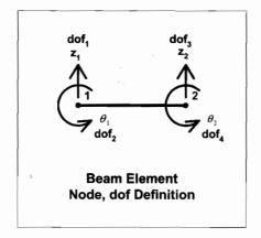
Figure 13.5: Beam element node and degree of freedom definition.
