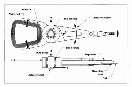
Figure 17.1: Drawing of actuator/suspension system.
