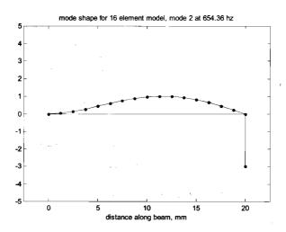
Figure 16.3: First bending mode, 654 hz.
