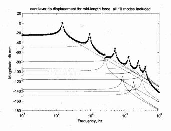
Figure 1.4: Individual mode contribution to overall frequency response.
