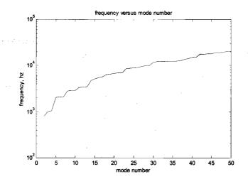
Figure 19.5: Frequencies versus mode number.
