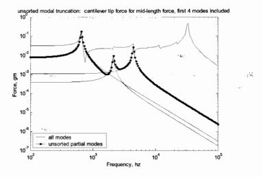
Figure 16.13: Overall plus individual mode contributions for the four unsorted mode model.
