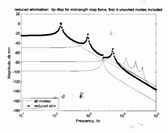
Figure 15.14: Cantilever tip displacement for mid-length force, first four modes included – unsorted modal truncation, modred "del" option.
