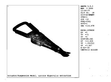
Figure 17.25: Mode 18 mode shape plot, 6561 hz.
