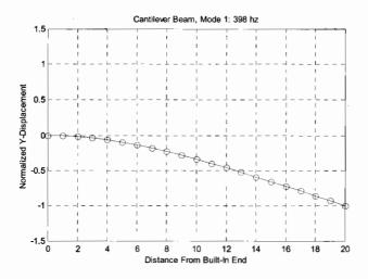
Figure 14.2: Cantilever beam first mode.
