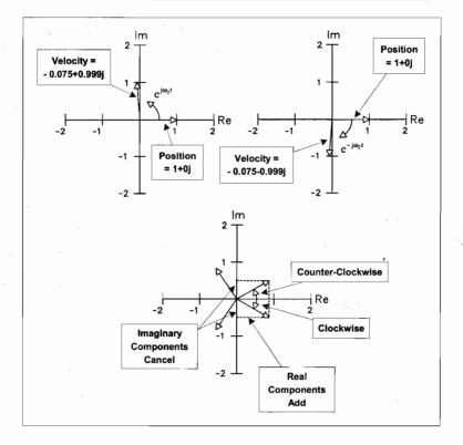
Figure 5.4: Argand diagram explanation.
