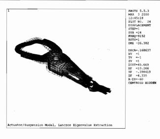
Figure 17.26: Mode 24 mode shape plot, 9152 hz.
