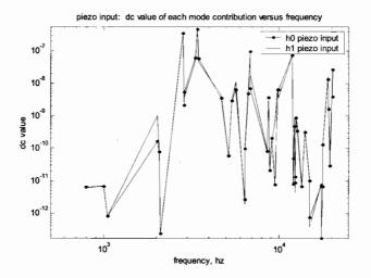
Figure 19.26: dc gain versus frequency for both heads for piezo input.
