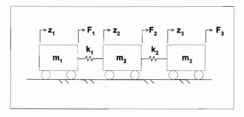
Figure 8.1: tdof undamped model for modal analysis.
