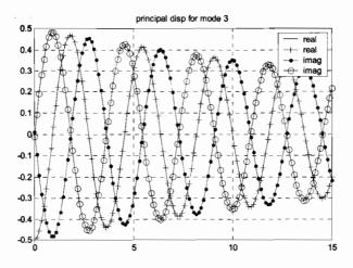
Figure 10.11: Principal real and imaginary displacements, mode 3.
