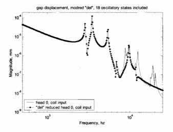
Figure 19.52: Head 0, coil input, 18 reduced oscillatory states included.
