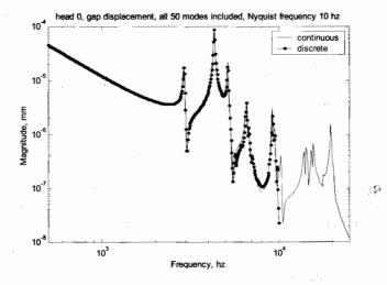
Figure 17.37: Discrete system frequency response overlaid on continuous system, sample rate 20 khz, Nyquist frequency 10 khz.
