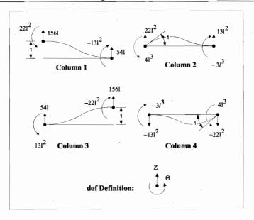
Figure 14.1: Beam element consistent mass matrix terms.
