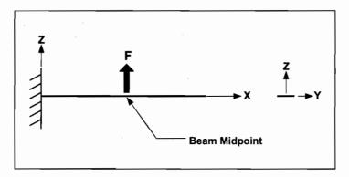
Figure 15.1: Cantilever beam with forcing function at midpoint.
