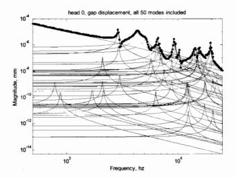
Figure 17.36: Head 0 frequency response, overlay of individual mode contributions, 50 modes included, non-uniform damping with zeta = 0.005 for all modes except modes 11, 12 and 13, which have zeta = 0.04.
