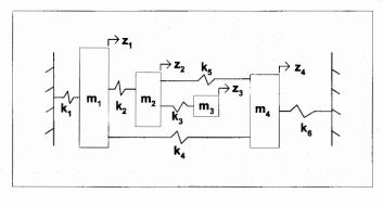
Figure P2.1: four dof system.
