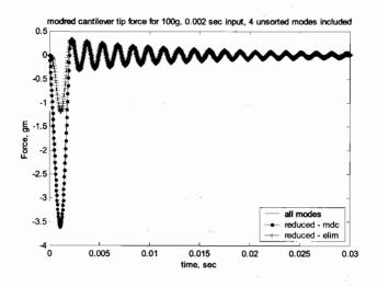
Figure 16.18: Half-sine shock pulse response for full, reduced unsorted "mdc" and reduced unsorted "del" models.
