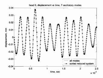
Figure 18.21: Impulse response comparisons for oscillatory system, full model (all oscillatory modes) and sorted reduced system with seven oscillatory modes.
