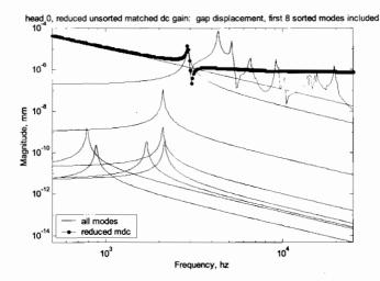
Figure 17.43: Unsorted Reduced "modred" matched dc gain frequency response, first eight unsorted modes included, showing overlay of eight individual modes.
