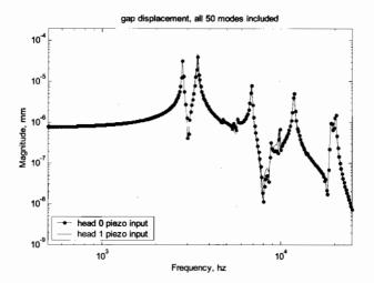
Figure 19.8: Piezo input frequency response from MATLAB, zeta = 0.005.
