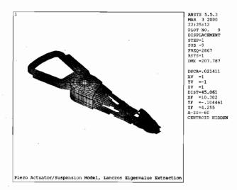
Figure 19.16: Mode 9, 2867 hz, suspension torsion, out of phase.
