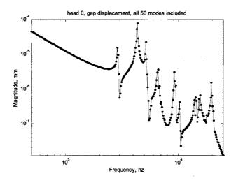
Figure 17.14: Frequency response for head 0 for coil input.
