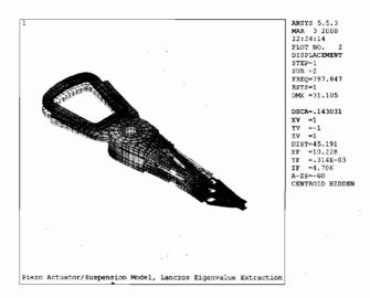
Figure 19.10: Mode 2, 798 hz, actuator pitching mode.
