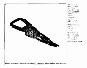
Figure 19.21: Mode 21, 6822 hz, suspension/arm lateral out of phase.
