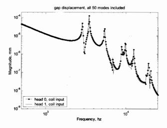
Figure 19.7: Coil input frequency response from MATLAB, zeta = 0.005.
