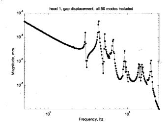
Figure 17.15: Frequency response for head 1 for coil input.
