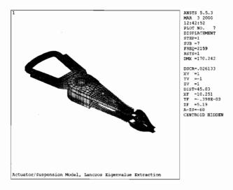
Figure 17.20: Mode 7 mode shape plot, 2159 hz, suspension bending modes.
