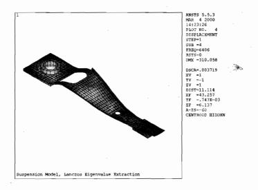
Figure 17.7: Mode 4, 6406 hz, second bending mode.
