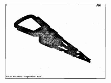
Figure 19.2: Complete piezo actuator/suspension model.
