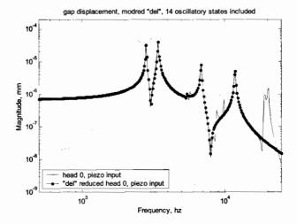
Figure 19.49: Head 0, piezo input, 14 reduced oscillatory states included.
