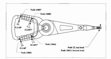
Figure 17.12: Nodes used for reduced MATLAB model. Shown with partial finite element mesh at coil.
