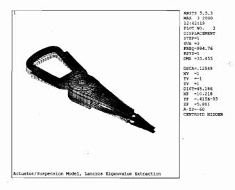
Figure 17.18: Mode 3 mode shape plot, 885 hz, coil and bottom arm bending.
