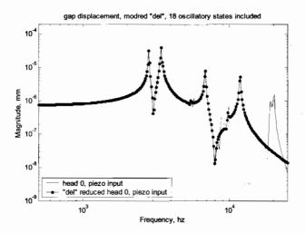
Figure 19.53: Head 0, piezo input, 18 reduced oscillatory states included.
