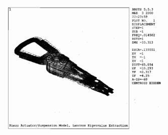
Figure 19.9: Mode 1 undeformed/deformed plot, 0.014 hz, rigid body rotation.
