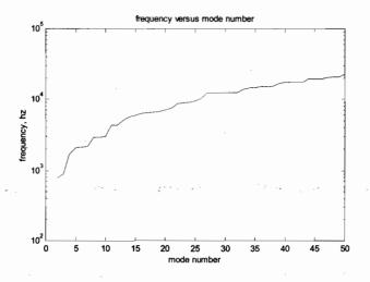
Figure 17.13: Frequencies versus mode number.
