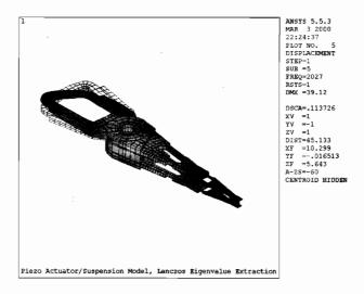
Figure 19.13: Mode 5, 2027 hz, actuator/coil torsion about x axis.
