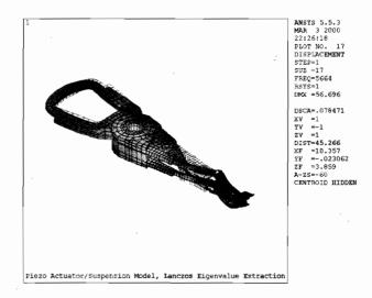
Figure 19.20: Mode 17, 5664 hz, piezo bending, arm tip torsion, coil bending.
