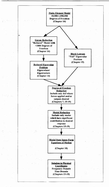
Figure 1.3: Model size reduction flowchart.
