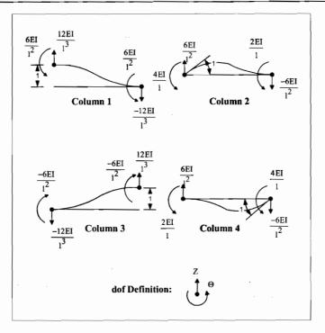
Figure 13.4: Beam element stiffness matrix terms.
