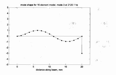
Figure 16.4: Second bending mode, 2120 hz.
