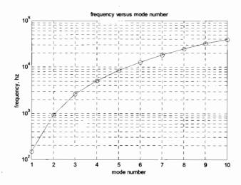
Figure 15.4: Resonant frequency versus mode number.
