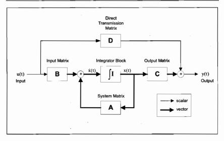
Figure 15.13: State space system block diagram.
