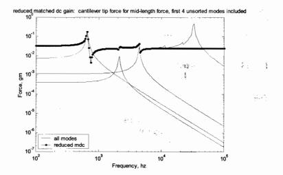
Figure 16.17: Overall frequency response with overlaid individual mode contributions for unsorted "mdc" modred option, with the 12 highest frequency modes reduced.
