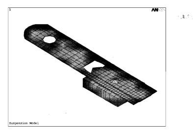
Figure 17.3: Flexure and recording head (slider) portion of suspension. Note the "dimple" at the center of the slider, a point about which the slider rotates to comply with the disk topology.
