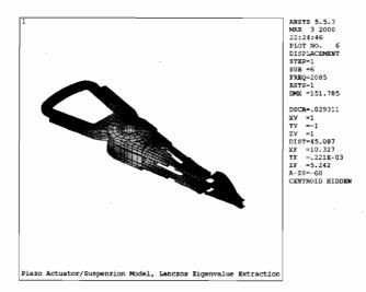
Figure 19.14: Mode 6, 2085 hz, suspension bending mode, some arm interaction.
