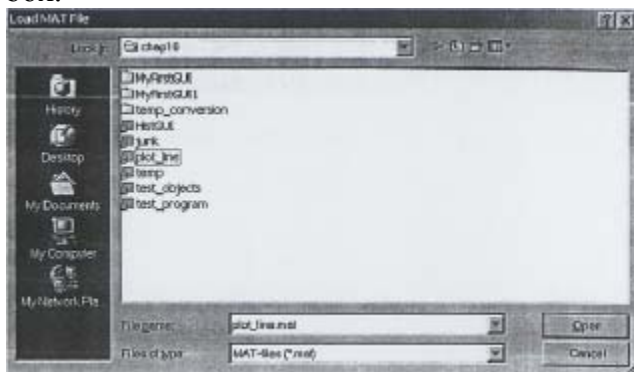
Figure 1.27 A file open dialog box created by uigetfile on a Windows 2000 Professional system.
