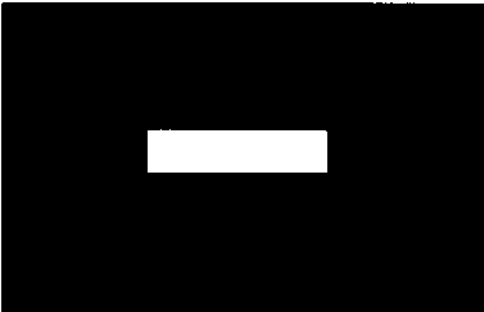
FIGURE 11.2A The rectangular object (2 pixels by 10 pixels) used in Example 11.1. The Fourier transform of this image is shown in Figure 11.2B and C.
