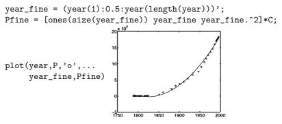
This technique can be used to fit any function that is linear in its parameters. (MATLAB provides the functions polyfit and polyval as easy interfaces to the functionality that we have just illustrated using matrix multiplication and division.)
