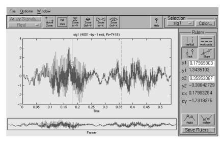
Here you have a plot of the time series with two "rulers". The rulers can be used to pick values out of the data, as well as to calculate intervals and slopes. The data in the **Rulers** box at the right of the display shows this information. At the bottom is a "panner". If you click on the **Zoom In-X** button a couple of times, the top plot shows an expanded portion of the data, and the panner at the bottom shows the location of the top box within the entire signal.
