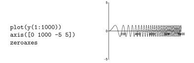
The frequency content of this signal as a function of time can be calculated using the **specgram** function. This function uses the Short Time Fourier Transform (STFT) technique. The STFT chops up the signal into a series of short segments and calculates the FFT of each segment. Each FFT becomes the estimate of the frequency content at that time. For our example we can get a quick display by typing:
