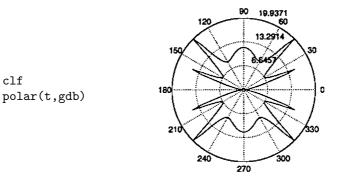
In this case you must use a modified version of **polar** that interprets a zero radius as a 0 dB value which should go at the outer limit of the plot. Negative decibel values should appear at smaller radii. I have implemented these ideas in the m-file **negpolar** (see companion software):
