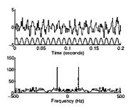
The top trace in the top plot is the noisy data, and the bottom trace is the original pure sinusoid. The lower plot clearly shows the frequency at 100 Hz.
