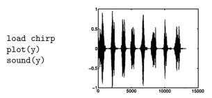
The volume of the sound can be controlled from within MATLAB using the soundsc function and supplying an upper and lower limit. Or if you wish, you can use your computer's system software to control the volume. On UNIX the volume of the sound can be controlled with the audiotool. On a PC the volume can be controlled from the "properties" panel of the sound recorder.
