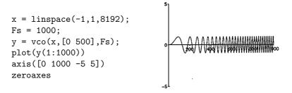
We used the axis command to set the y-axis limits to [-5 5] instead of the default limits, in this case, of [-1 1]
