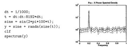
The frequency scale is normalised to the Nyquist frequency. The middle line is the PSD estimate and the two dashed lines are the 95% confidence intervals. Typing help spectrum reveals that there are many parameters that you can adjust when calculating the power spectrum. MATLAB's spectrum function uses the Welch method of PSD estimation,<sup>6</sup> which divides a long signal into a number of smaller blocks, calculates
