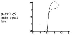
This is an improvement, but we still do not know where the aircraft started, where it finished, and how it went in between. We can see an animation of the trajectory by typing: comet(x,y)
