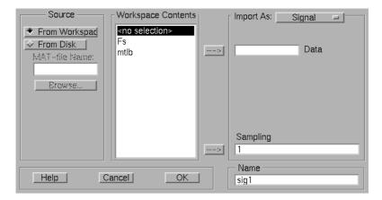
Click on the variable mtlb and the arrow button (-->) to get mtlb to appear in the Data box (or just type mtlb there). Do the same to make Fs appear in the Sampling box. Then press OK. A signal called sig1 appears in the Signals box in the main SPTool panel. Clicking on the View button at the bottom of the Signals box opens the signal browser panel:
