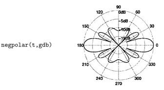
The negpolar function also omits the solid outer circle which, like the box drawn around MATLAB's default plot output, unnecessarily frames the plot and can obscure the data that you are trying to display. A faint dotted grid is enough to put the plotted points in context. I will say more about this in the section on Handle Graphics later (see page 65).
