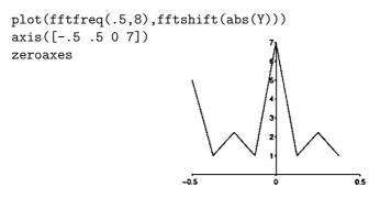
Let us do a slightly more realistic example. We simulate some data recorded at a sampling frequency of 1 kHz, corresponding to a time step dt = 1/1000 of a second. The Nyquist frequency is, therefore, 500 Hz. Suppose there is a 100 Hz sinusoid contaminated by noise. We simulate the data, calculate the FFT, and plot the results as follows:
