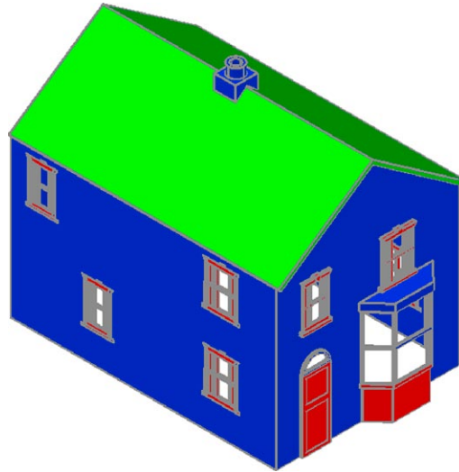
Fig. 16.17 First example – a Realistic view of the assembled walls, windows, bay, roof and chimney
