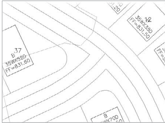
Figure 12.9 Completed feature line Trim and Break commands
