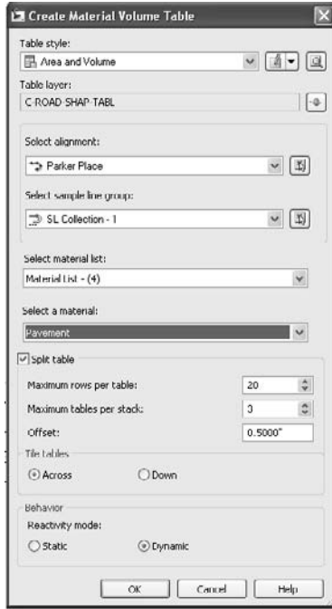
Figure 11.31 Assign Pavement for the first table.
