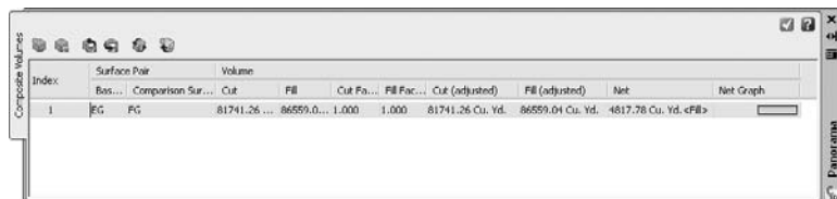
FIGURE 5.37 Composite volume calculated
