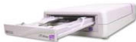
**CD-RW** Refers to the ability to read and write multiple times onto a CD.
