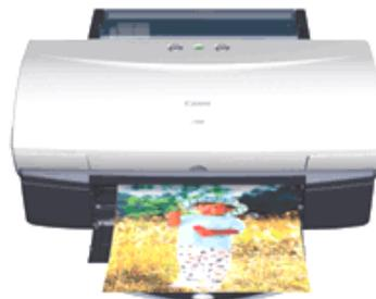
Bubble jet printers, like ink jet printers, have an average of 64 nozzles and are capable of producing 300 to 1200 dpi resolution. Black-and-white and color bubble jet printers are available.
