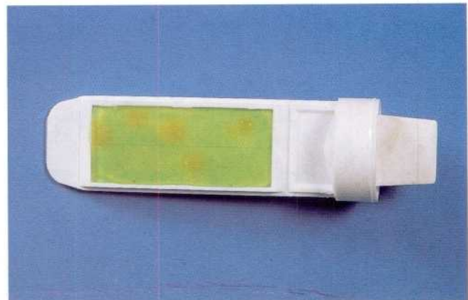
17 Dipslide. The dipslide is a way of collecting and transporting urine specimens to the laboratory. The dipslide is dipped into the urine and the excess allowed to drain. The dipslide is then placed in its plastic container and transported to the laboratory for incubation. The number of colonies can be used to determine whether the organisms are present in significant numbers.
