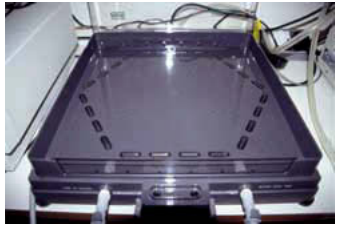
Figure 17.18 Pulse-field gel electrophoresis (PFGE) equipment. In this technique an electric current is passed through the gel in timed pulses at differing angles to separate very large DNA molecules. Note the hexagonal arrangement of the electrodes in this case
